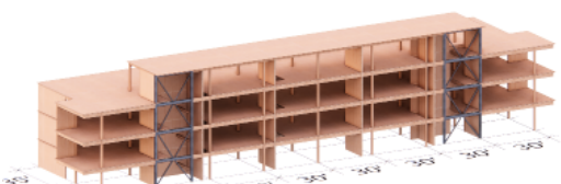
Vertical, horizontal, and bracing and CLT structure
