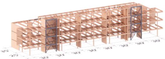
Vertical, horizontal, and bracing structure
